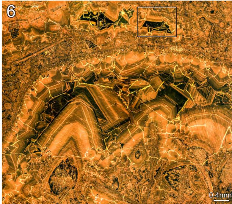
Fig. 6 --- CL image from same area as Fig. 5; shelter cavity cements showing multiple orange to black luminescent zoning.
