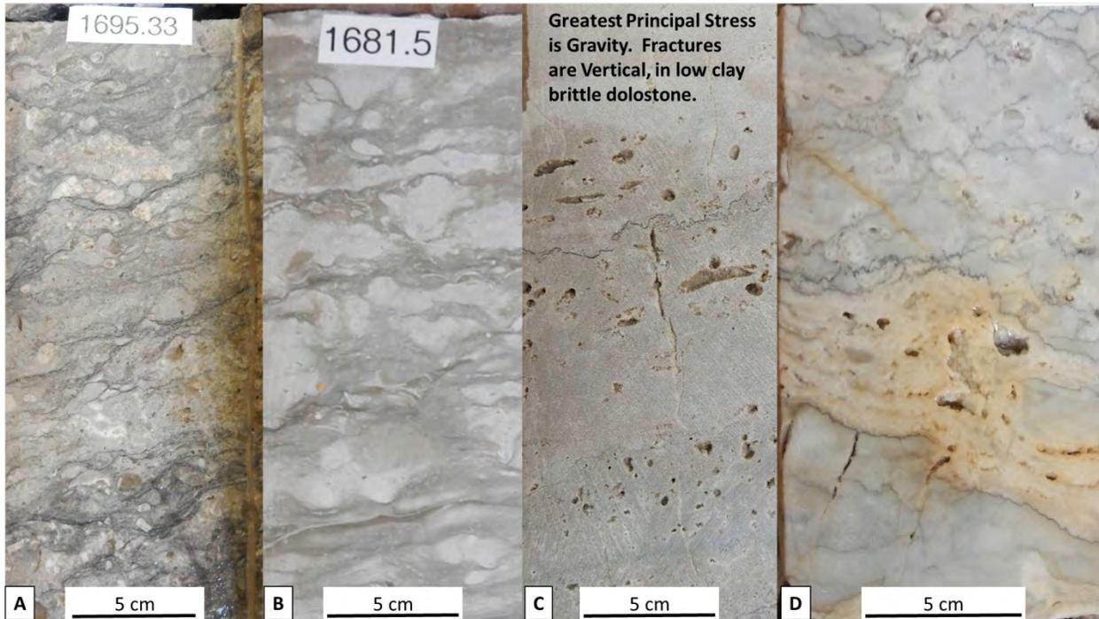
FIG. 23. – **A)** and **B)** Argillaceous dolostones show significant ductile deformation. **C)** and **D)** Pure Dolostones with low clay content do not show ductile deformation. Uneven flexing along stylolites produces brittle fractures. Gravity provides the greatest principal stress, which is vertical compression.
