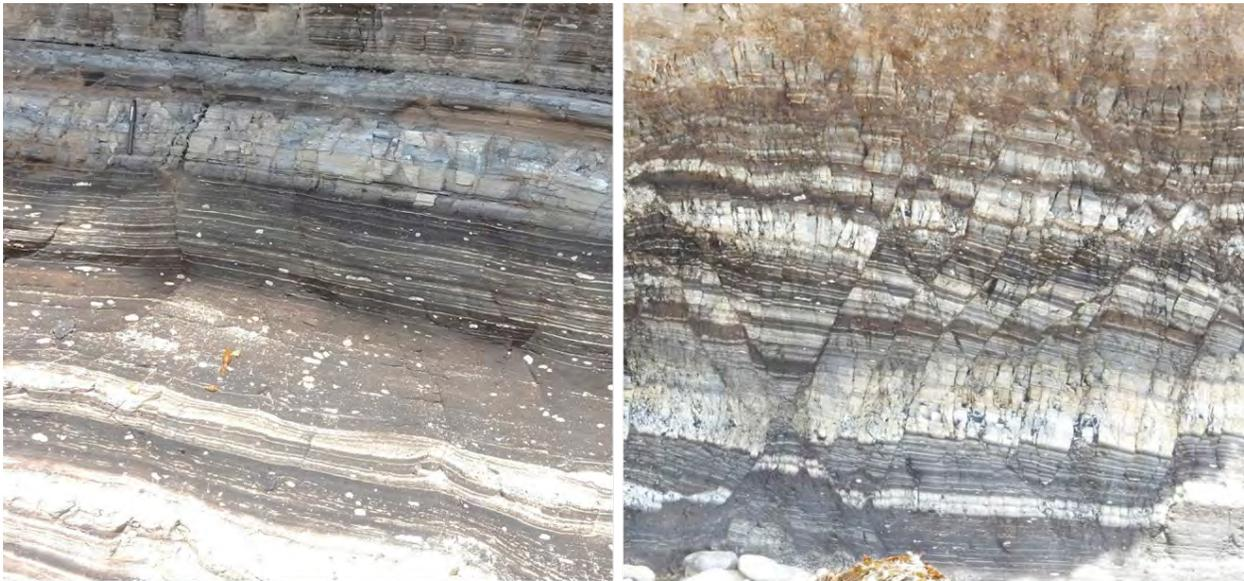
**TOC in Monterey Shales ranges from 5% to over 25%. High Kerogen Content correlates with low strength.**
