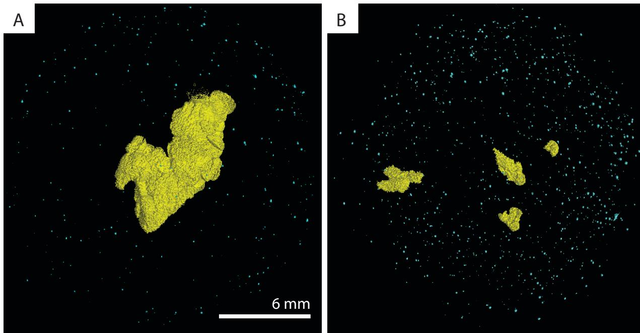
**SUPPLEMENTARY FIGURE 1**—3D CT scan reconstruction of mineral precipitation experiments. Yellow is remaining fish tissue, blue is glass beads cemented together by authigenic mineral precipitation. Scale bar refers to both.
