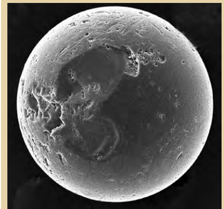
Figure 13. SEM image of glass bead with divots, conchoidal spall pits, and scratches.
