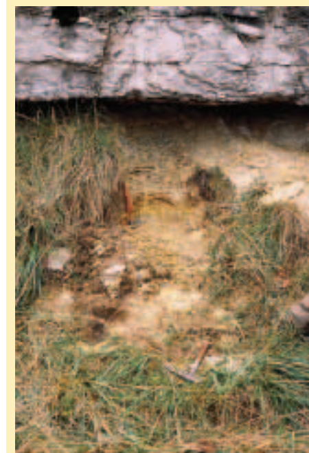
Figure 1: Outcrop of the Millbrig K-bentonite along U.S. Highway 68 at entrance to Shakerstown, Kentucky. The ash bed is about 70 cm thick at this section. Head of top hammer marks the base of the bed.
